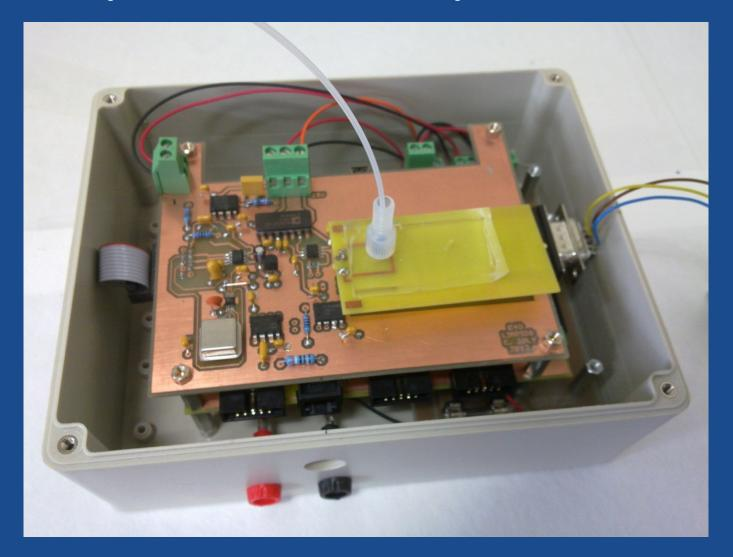
University of Hull: Detection chip and baseline suppression board
