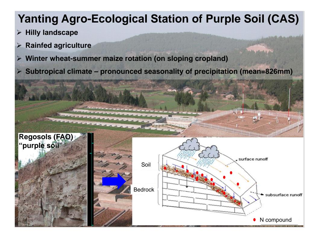
Large free-drain field lysimeters (area: 4m × 8m)
