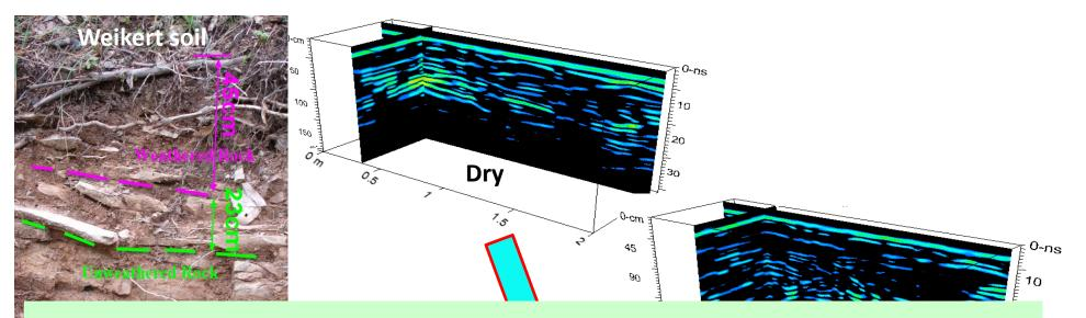
Time-lapsed GPR in combination with real-time soil water monitoring have revealed flow paths in .... fractured shales and the impacts of soil layering on subsurface lateral flow
